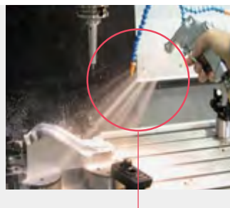
Coolant Gun Coolant gun helps keeping the work environment clean.
